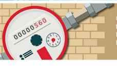
Check your water meter before and after a two-hour period when no water is being used. If the meter changes at all, you probably have a leak.
